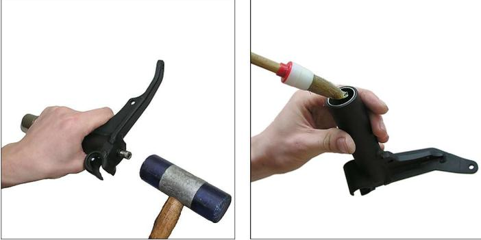
4. Remove the hex bolt **A** and slide the stanchion tube **3** (golden) out of the knuckle.
